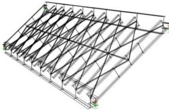
Fig. 1. SAP2000 model of grandstand steel structure.
